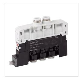
Activation Electrically Working pressure min./max. 3 ... 8 bar 5 ... 50 °C Ambient temperature min./max. Medium temperature min./max. 5 ... 50 °C Medium Compressed air 40 µm Max. particle size Oil content of compressed air 0 ... 5 mg/m<sup>3</sup> Nominal flow Qn 610 l/min Protection class with connection IP65 100 % Duty cycle
